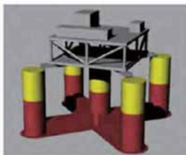
Figure 4/ United States Floating Substation Design Concept Diagram Source/ [10]
