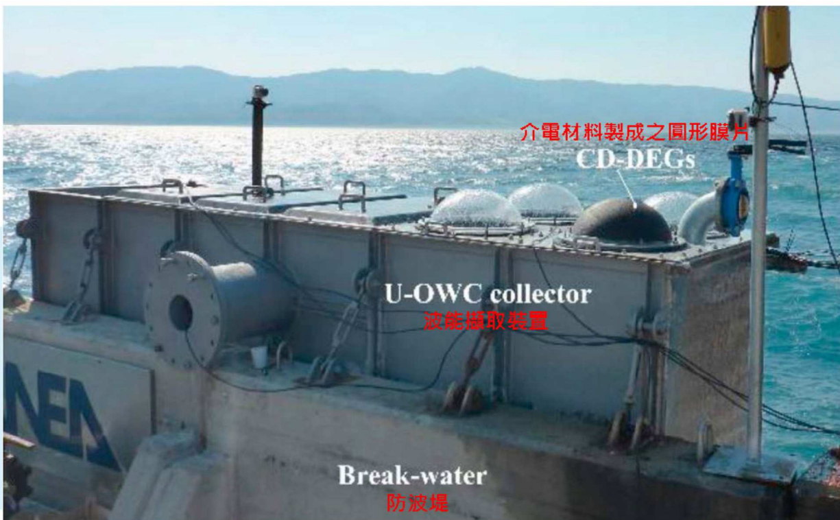
Figure 4/ Experiment using DEG in the breakwater-integrated OWC wave energy converter Source/ Moretti et al. 2020
