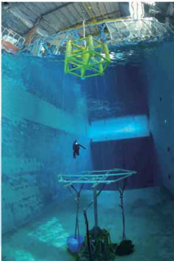
Figure 2/Testing of the floating wind platform in the deep-water basin at Ifremer Image by Ifremer/ O.Dugormay
