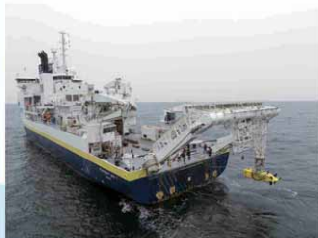
Figure 3/ Launch of the AUV 6000 Ulyx from R/V Pourquoi Pas? The Ulyx has a capacity to dive down to 6,000m depth and to accomplish a mission up to 48 hours of autonomy Image by Ifremer, S. Lesbats (2022)
