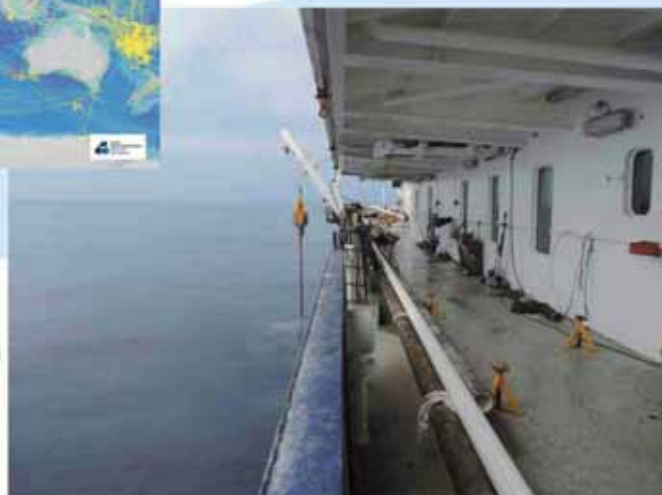
Figure 5/ Giant coring system in action from the R/V Marion Dufresne ( https://www.flotteoceanographique.fr/en/Facilities/Tooling/Sediment-Sampling/Gravity-Corer )
