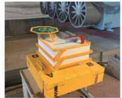
Figure 5/ Taiwan Floating Substation Model Diagram Images by Department of Hydraulic and Ocean Engineering, National Cheng Kung University
