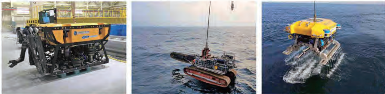
Figure 2/ Development of KIOST's underwater construction robots in Korea (URI-L · URI-T · URI-R)
